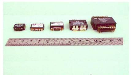
Picture 1: Transformers of Various core sizes: 20, 32, 40, 55 and 80 (left to right).
