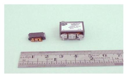
Picture 2: A pre-magnetizing choke of 0.33  $\mu$ H\40 Adc (left), compared to a regular choke of 0.4 $\mu$ H\40Adc (right).
